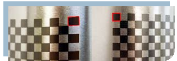
f.l.t.r. stainless steel tube mark of uncalibrated system; stainless steel tube mark of calibrated system
