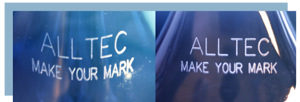
f.l.t.r. PET bottle mark of uncalibrated system; PET bottle mark of calibrated system
